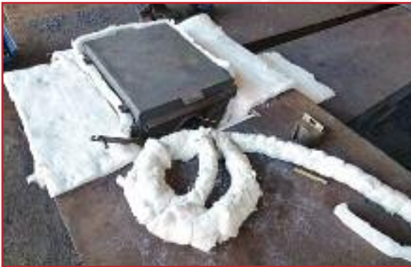
Prepared test slab with thermocouples and data logger is about to enter the furnace
