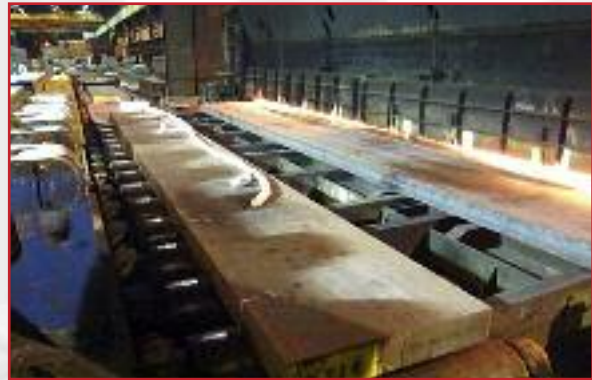
Prepared test slab with thermocouples and data logger is about to enter the furnace
