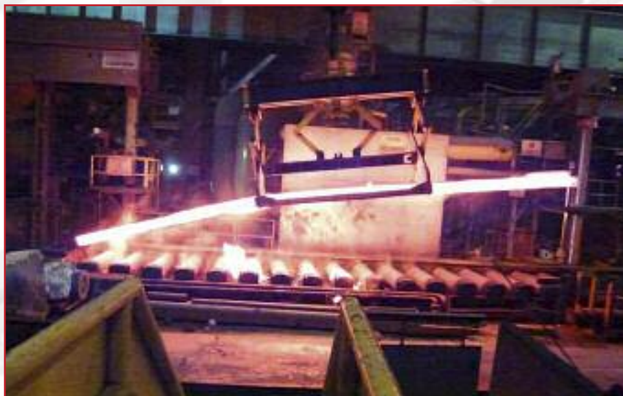
The test slab gets taken off the hot roller table to remove the measurement equipment
