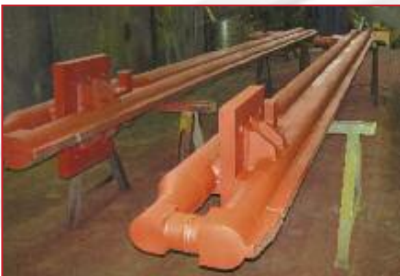
Prefabrication of skid pipes
